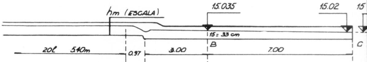
PERDIDA DE CARGA ENTRE LOS PUNTOS B Y C  $W = 0.33$   $Q = 0.132 \text{ m}^3/\text{s}$   $f = 1.06 \text{ m}$
